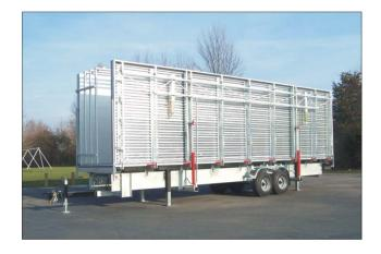
To Lower the first deck wing by using the push-button remote control pendant to release hydraulic cylinder.
